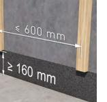
The battens should be positioned 10 mm higher than the recommended clearance and 20 mm down from the soffit/window cill to accommodate the 10mm drip edge to the weatherboard.
