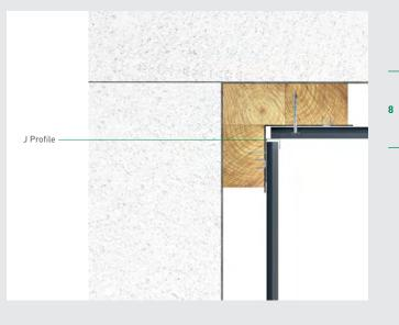
Window Details with Hardie® VL Plank weatherboard on edge
