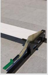
When using the Hardie<sup>™</sup> Guillotine cutting tool, the painted face of the board must be upward facing.
