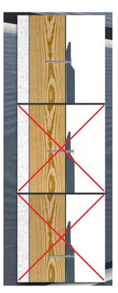
Fix through the tongue part of the weatherboard 25 mm down from the top edge. When fixing the ends of the cladding, ensure the fixing is placed 15 mm in from the edge.
