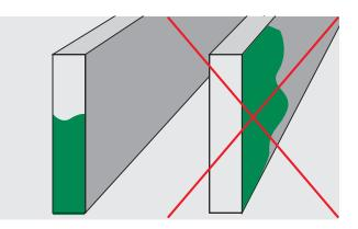
Along with cut edges, Hardie<sup>™</sup> Seal edge coating will need to be applied to any exposed back edges of the boards. This is common when using Hardie<sup>®</sup> Plank weatherboard on edge into window/door reveals. Hardie<sup>™</sup> Seal edge coating may also be used to deal with small scratches and marks less than 6 mm along with any exposed fixing heads. It should be used sparingly and only on the affected area otherwise it may become visible.
