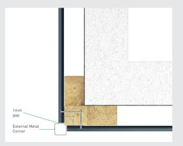
When installing the 2-Part VL Corner Profile below, screw the inner section over the cladding, with the Hardie™ Plank screw, and then click the outer section into position. One fixing will need to go through the outer trim to be sure it stays in line. It is recommended this goes at the top, out of eye line.
